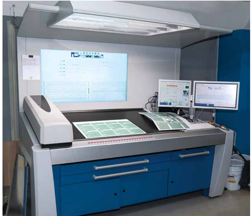
Right: Identical to the larger Rapida presses: The console of the Rapida 75 PRO
